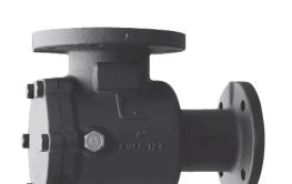
Grundfos Series SD, Suction diffuser provides and ensures a uniform flow pattern to the suction side of the pump ensuring a stable NPSH. Suction diffuser makes it possible to install the pump in a very narrow spacing as no long bends are necessary.
