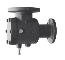
Grundfos Series SD, Suction diffuser provides and ensures a uniform flow pattern to the suction side of the pump ensuring a stable NPSH. Suction diffuser makes it possible to install the pump in a very narrow spacing as no long bends are necessary.
