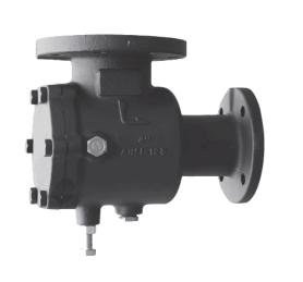
Grundfos Series SD, Suction diffuser provides and ensures a uniform flow pattern to the suction side of the pump ensuring a stable NPSH. Suction diffuser makes it possible to install the pump in a very narrow spacing as no long bends are necessary.
