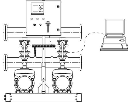
System with external controller (open loop)
